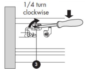
Insert the screwdriver in the cross slot and lift up the flap
