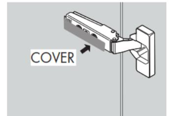
After adjustment, fit the Ab covers onto the other hinges
