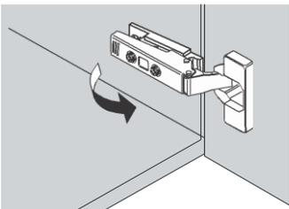
Squeeze the flap at the rear of the hinge and pull forward. Never remove the hinge plates that are screwed onto the carcass
