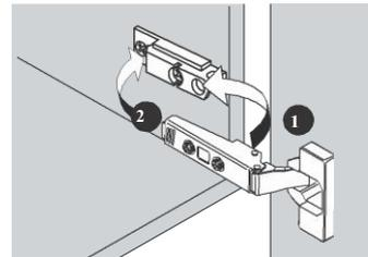
Align the bar on the hinge into the groove in the plate (1) and clip the hinge backwards into position (2)
