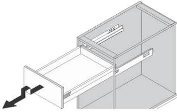
Pull; when it is fully open lift and continue to pull gently, following the movement of the arrow.
